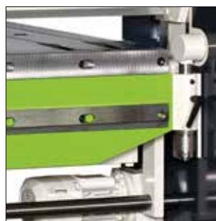
Compact folding beam, only 280 mm (11"), grants easy and ergonomic work at the machine.
