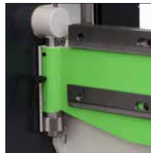
Compact folding beam, only 300 mm (11.8"), grants easy and ergonomic work at the machine.
