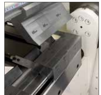
CNC adjustment of folding center, sheet thickness and crowning.
